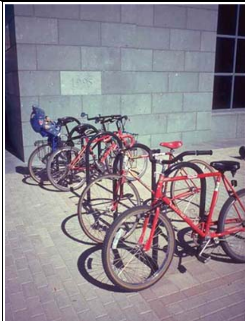
The Denver standard inverted U type bike rack solves contemporary bicycle parking"
