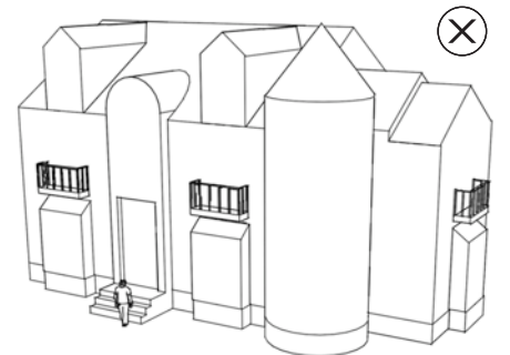
89. Avoid using a significantly higher number of building forms than are typically seen in the surrounding historic context. This can cause a building to appear busy and overly massive.
