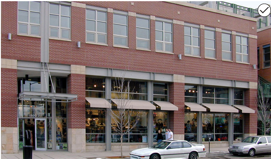
101. Wrap a parking structure or stack it above retail or other active uses at the street level.
