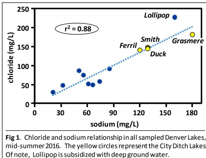
**Fig 1.** Chloride and sodium relationship in all sampled Denver Lakes, mid-summer 2016. The yellow circles represent the City Ditch Lakes. Of note, Lollipop is subsidized with deep ground water.
