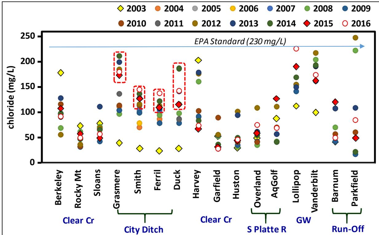
**Fig 2.** Chloride levels in Denver Lakes, 2003-2016. Source water is delineated in blue below lake designations. The red dashed rectangles delineate the past 5 years of data in the City Ditch Lakes, which received recycled water from 2004 – 2016.
