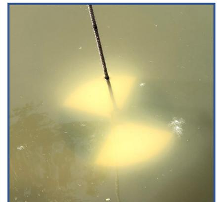
**Fig 3.** Secchi disc from mid-lake (7/12/18) at six inch depth.
