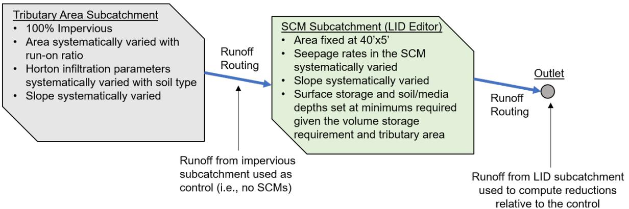
**Figure A.03.2.2: Graphical guide showing the subcatchment layouts and design variables**
