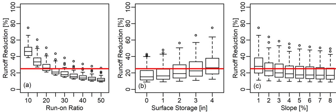
Figure A.03.2.7: Effectiveness curves generated from outputs of SWMM analysis for Level 3
