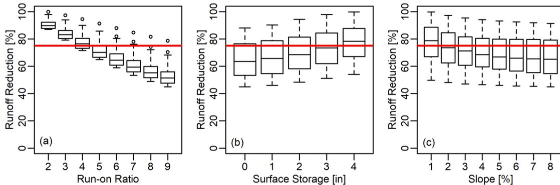
Figure A.03.2.5: Effectiveness curves generated from outputs of SWMM analysis for Level of Green 2
