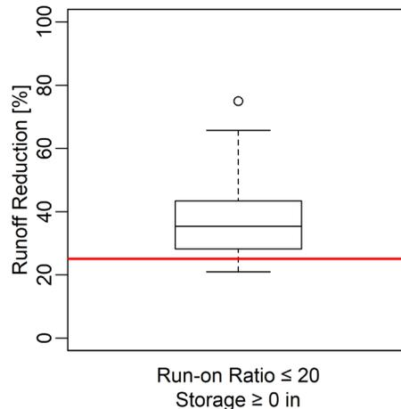
Figure A.03.2.8: Boxplot showing that 75% of the simulations are above the runoff reduction threshold of 25% if the design criterion is met for Level of Green 3
