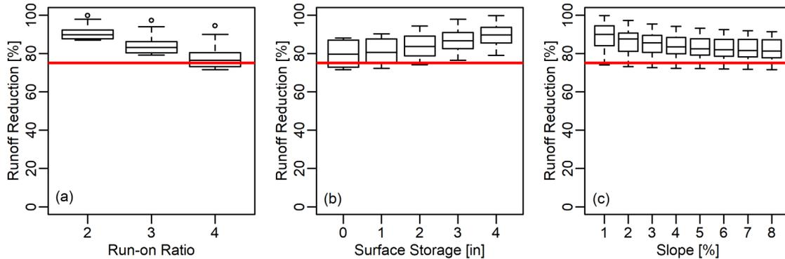
Figure A.03.2.3: Effectiveness curves generated from outputs of SWMM analysis for Level of Green 1
