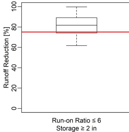
Figure A.03.2.6: Boxplot showing that 75% of the simulations are above the runoff reduction threshold of 75% if the design criteria are met for Level of Green 2
