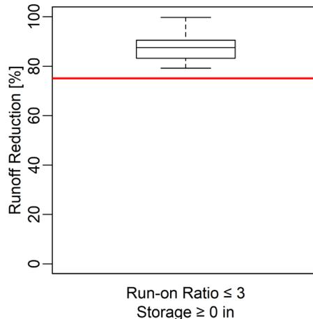
Figure A.03.2.4: Boxplot showing that >75% of the simulations are above the runoff reduction threshold of 75% if the design criterion is met for Level of Green 1
