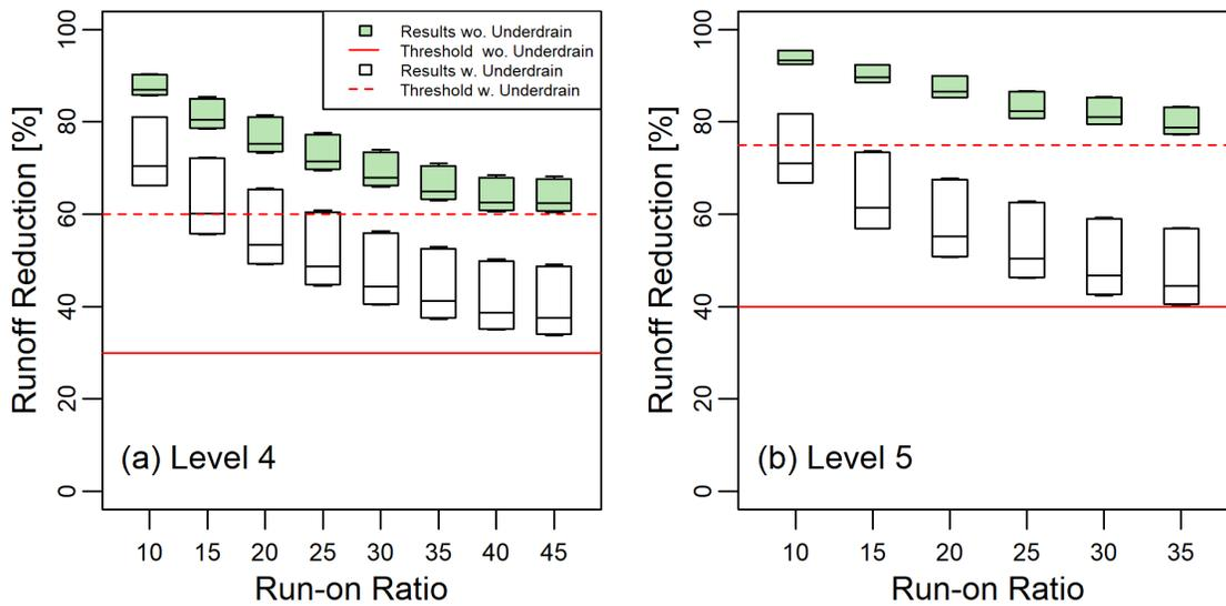
Figure A.03.2.9: Effectiveness Curves for Levels of Green 4 and 5. Variability in the boxplot is due to soil and slope.
