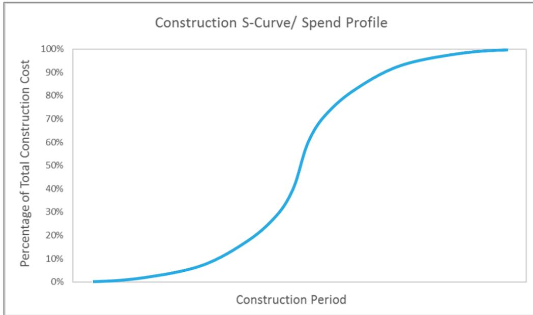
Figure 4: Sample construction S-curve — for illustration only
