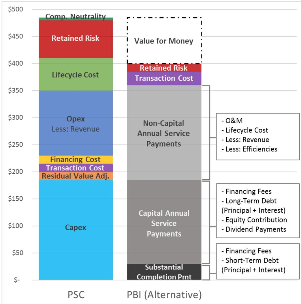
Figure 7: PSC and PBI Model comparison, Method 1 — for illustration only
