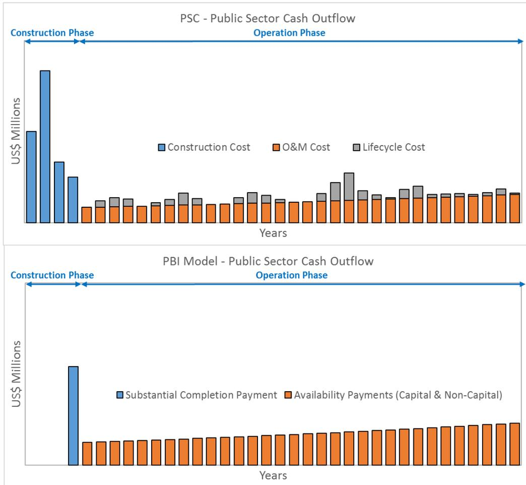
Figure 6: Comparison of sample cash flow profiles for the example PSC and PBI Model
