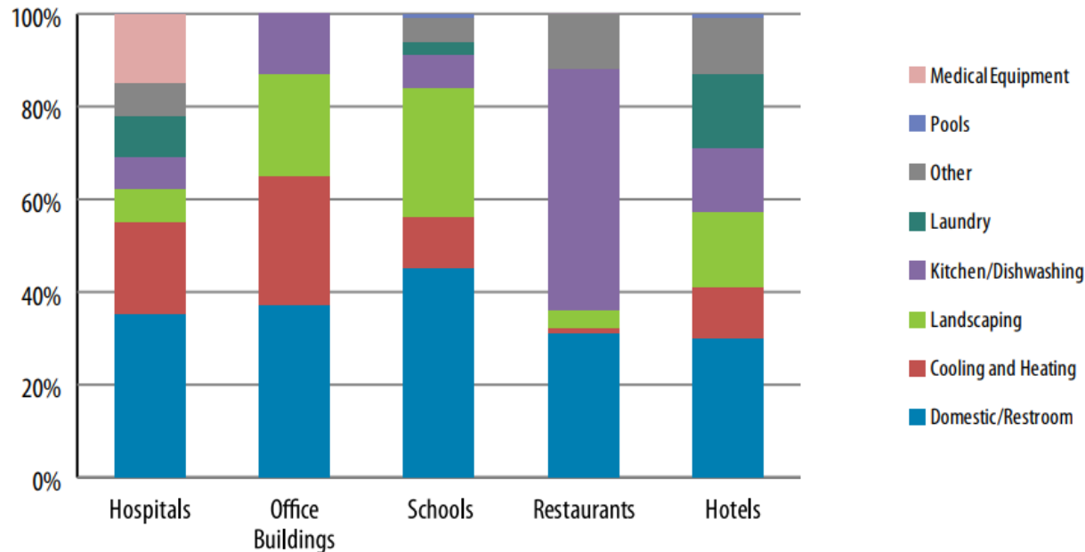
Figure 1-1. End Uses of Water in Various Types of Commercial and Institutional Facilities
