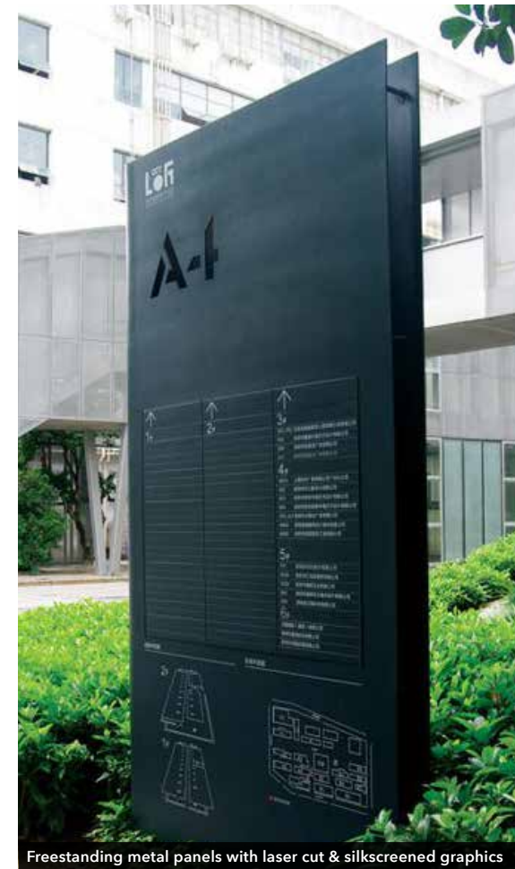
Freestanding metal panels with laser cut & silkscreened graphics
