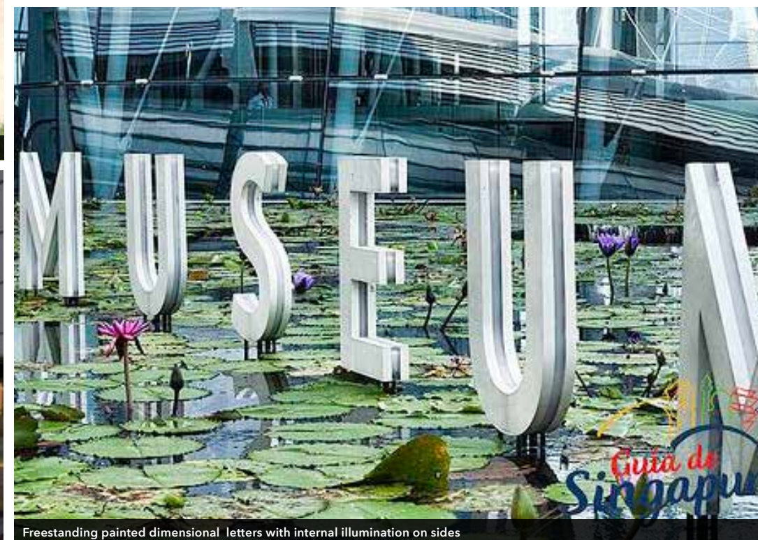
Freestanding painted dimensional letters with internal illumination on sides
