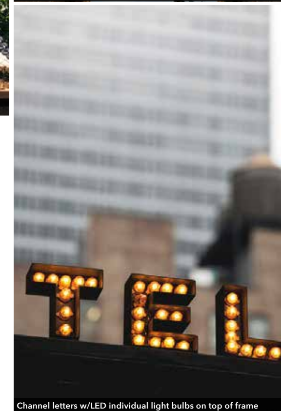
Channel letters w/LED individual light bulbs on top of frame
