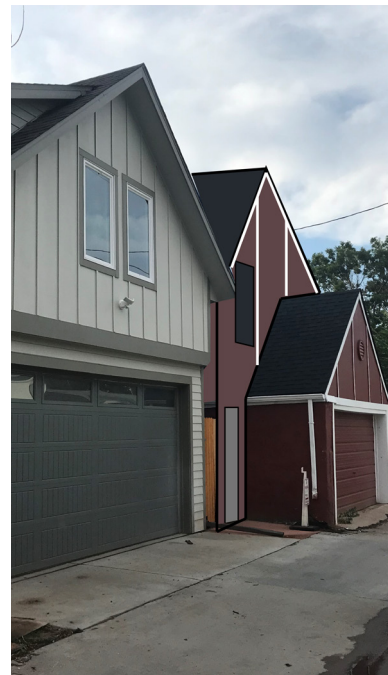
Under existing rules, the red garage in the left image could not be converted to an ADU as it does not have a 5' rear setback. The rendering of the red garage on the right shows an ADU addition meeting the minimum ADU setbacks.
