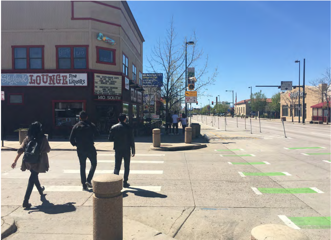
Green pavement markings and sign with supplemental flasher at Maple Ave.
