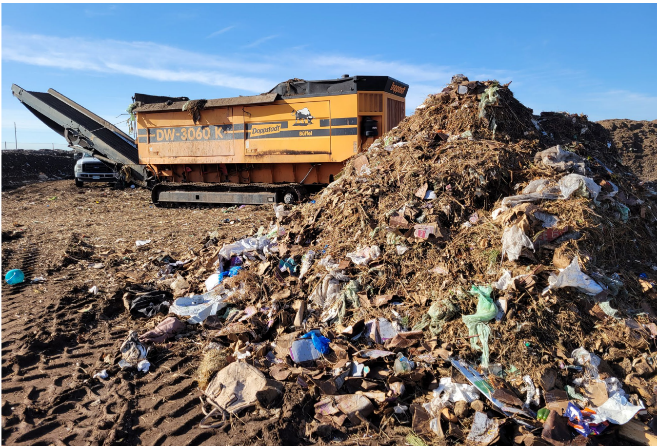
COLLECTED COMPOST | A load of compost waits to be processed at A1 Organics’ facility. Machines remove prohibited items that cannot be composted, such as plastic bags, which would otherwise contaminate the compost.
