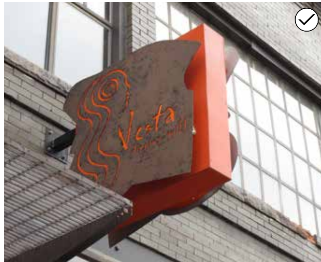
165. Use halo (left), push-through letters (right), LED and neon lighting (below) for signs when externally focused lighting is not possible.
