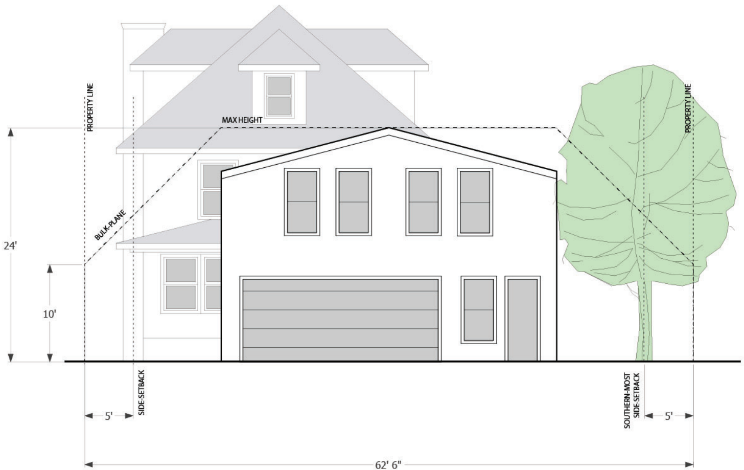
Elevation drawing of an ADU, showing the bulk-plane, height, and setback dimensions. Source: CPD
