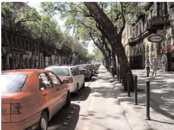
Along W. 17th Ave. explore new street cross-section alternatives to enhance the “green street” character and function. Investigate new ways to provide safe bicycle and pedestrian space, like a bike lane inside of the parking lane as pictured above.
